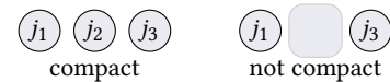
Figure 2-10: A compact level and one that is not because an unlabeled node appears between two nodes.
